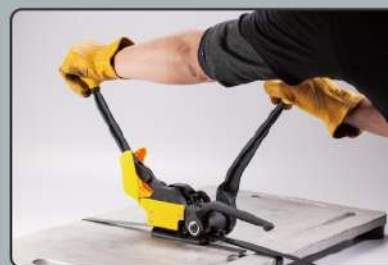
Seal and cut the strap
