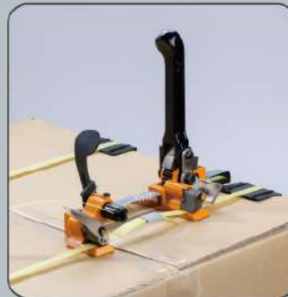
Tighten the strap and insert the seal
